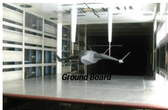
Gambar 2-2: Tes-setup model uji aerodinamik (LAGG, 2006)
