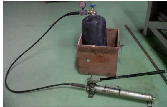
Gambar 2-3: Set up uji hydrostatic
