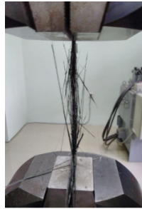
Figure 2-3: Testing Arrangement for Tensile Test Specimen
