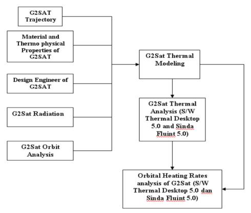
Figure 3-1: Orbital heating rates analyzing process of G2-SAT
