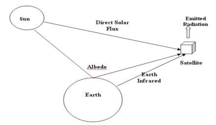
Figure 2-1: Thermal radiation environment for a typical spacecraft
