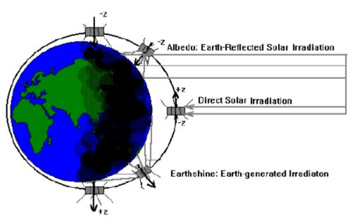
Figure 2-2: Three primary terms of the heat loads for calculating G2-SAT orbital heating rates
