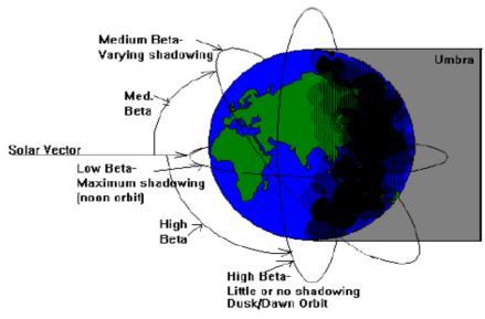
Figure 2-3: Beta angle in orbit duration
