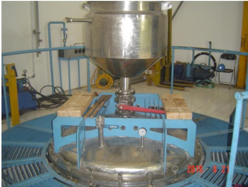
Gambar 3-3: Casting chamber
