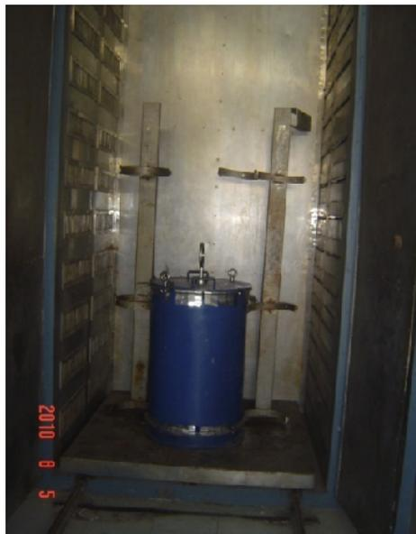
Gambar 3-4: Curing chamber
