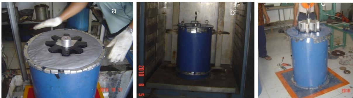
Gambar 3-7: Proses: coring (a), curing (b) dan decoring (c)
