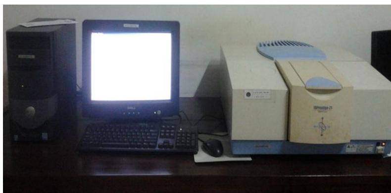
Gambar 2-1: Instrumen FTIR
