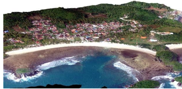
a) 3-Dimensional images of orthomosaic and DSM data
