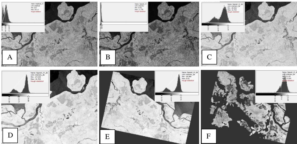
Figure 3-2: Pre-processing of SAR Sentinel-1 data, (A). The original format data that values was digital number, (B). Image after the radiometric calibration in the sigma\_0 format, (C). Image after the pixel value was converted to desibel (db), (D). Image after speckle filtering, (E). Image after geometric correction, (F). Image after subset or mask image
