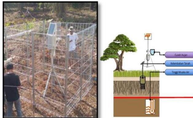
Figure 3-1: BRG's Peatland Water Monitoring System (Sipalaga) instrument that measures groundwater level, soil moisture and rainfall data for Sumatra and Kalimantan islands
