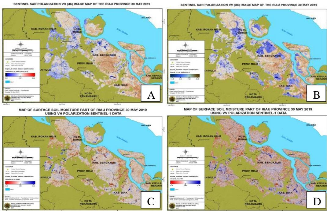
Figure 3-3: Image of SAR Sentinel-1 May 30, 2019: (A). polarization of VH Sigma\_0 format in decibels (db), (B). polarization VV Sigma\_0 format in decibels (db), (C). Polarization of VH as a result of Surface Soil Moisture (SSM) processing, and (D). Polarization of VV as a result of Surface Soil Moisture (SSM) processing
