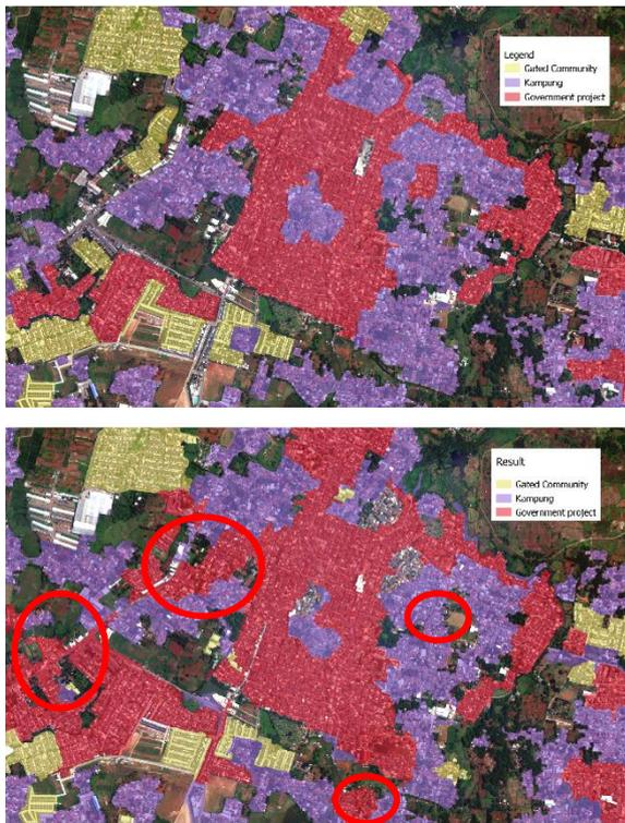
Figure 3-2: The reference map of housing types (above) and the result of classification using GEOBIA (under). Notice the difference highlighted by red circle.
