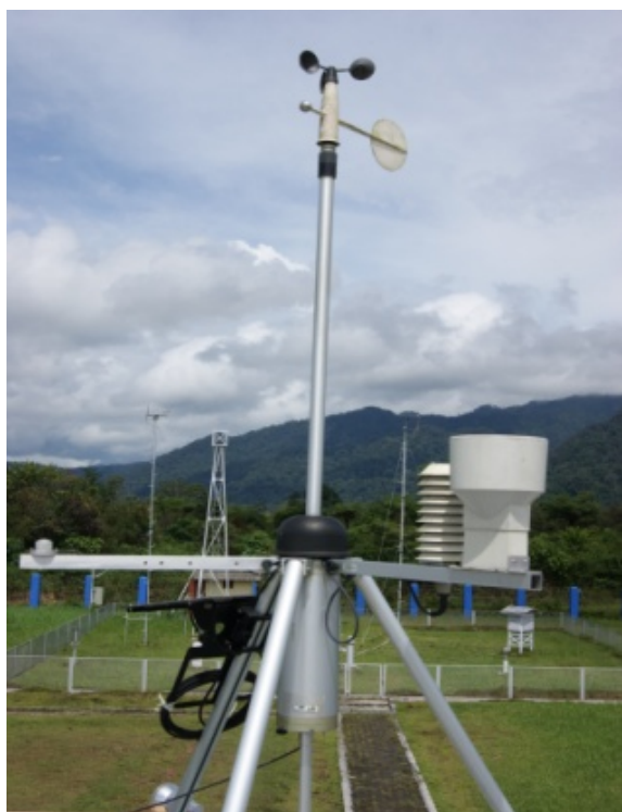
Gambar 3-3: Meteorological Automatic Weather Station (MAWS) Vaisala di Stasiun Pemantau Atmosfer Global Bukit Kototabang.
