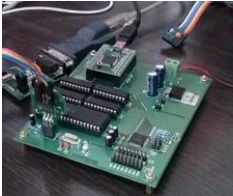
Gambar 2-3: Prototype 8 kanal USB Data Acquisition System (DAS)
