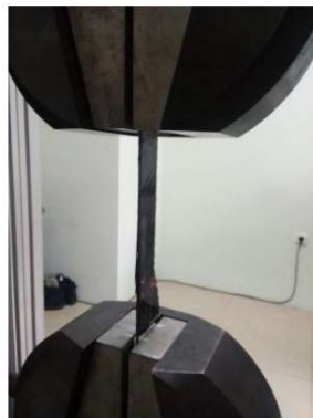
Figure 3-1: Tensile Test according ASTM D6641
