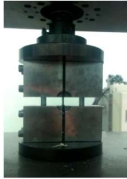
Figure 3-9: Compressive test ASTM D6641
