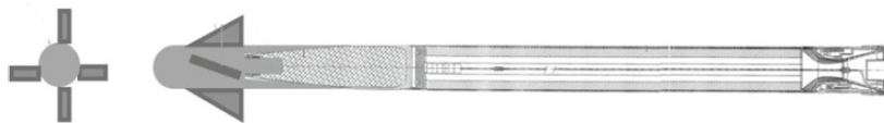
Figure 2-3: The 140 mm caliber rocket model in the research of (de Celis. 2017, 2018a) and (Lopez. 2019).
