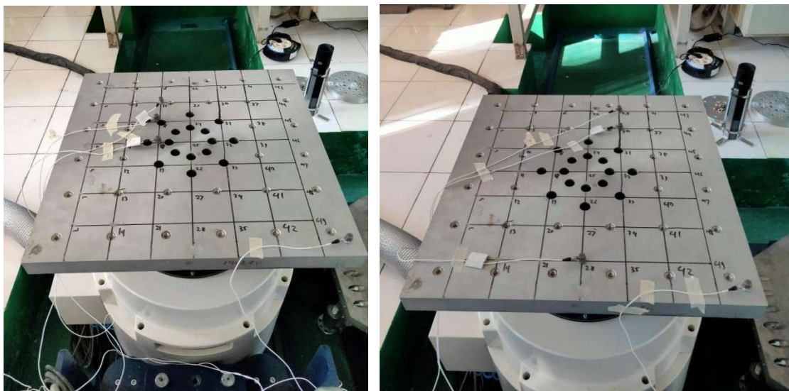
Figure 2-4: Accelerometer sensors set-up
