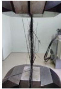
Figure 2-3: Testing Arrangement for Tensile Test Specimen
