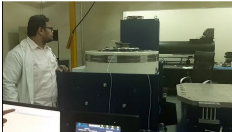
Figure 3-5: Testing of Wire Rope Isolation of RX 200 LAPAN Payload
