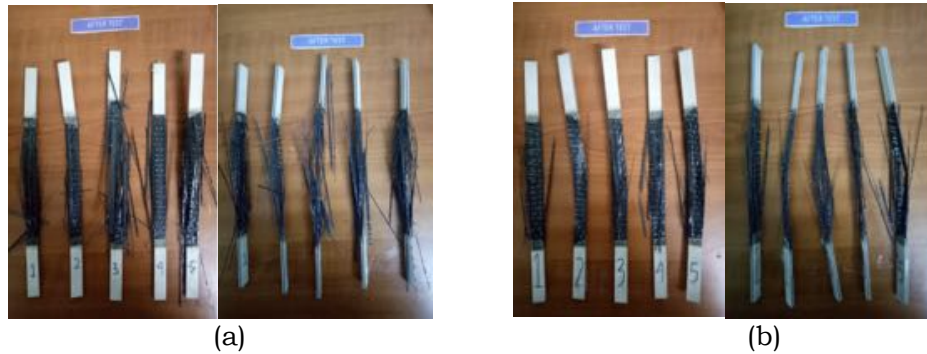
Figure 3-3: Composite Sample After Test (a) Non-Hole Composite (b) Open Hole Composite
