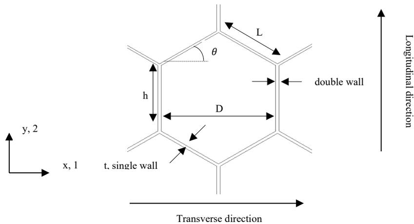
Figure 2-2: Details of 2D hexagonal honeycomb cell
