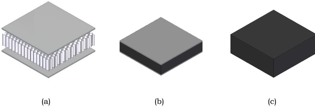
Figure 2-1: Honeycomb panel models for FEA (a) discrete model, (b) continuum model, (c) equivalent plate
