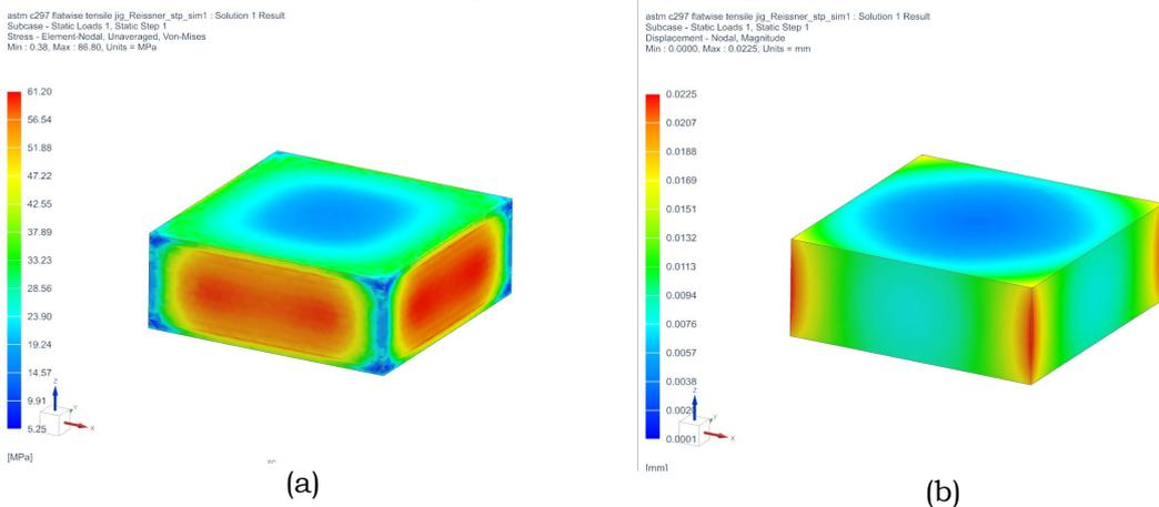
Figure 3-5: FEA of the flatwise tension test of Equivalent plate-Reissner Theories modeling (a) Stress, (b) Displacement
